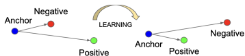
Figure 3. The Triplet Loss minimizes the distance between an anchor and a positive , both of which have the same identity, and maximizes the distance between the anchor and a negative of a different identity.
